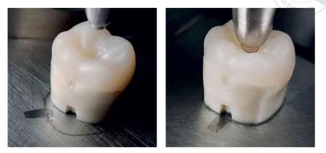
Fig 2 Base drawing used to guide the precise position of the specimen to initiate the vertical seating test.
